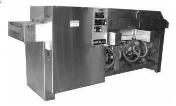
The PC3000 series post cleaning systems were designed to follow the Argus PC4700 and PC4800 series infrared fusing systems. The machine is designed to provide a flux removal with two stages of vigorous spray cleaning, mild brushing action followed by a fresh water rinse and turbo air drying. Board cleanliness is critical to quality PCB fabrication and the PC3000 series equipment is designed to deliver.
