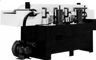
The PC6600 Series solder stripping systems were designed to precede Argus PC4700 and PC4800 series infrared fusing systems. The machine is designed to strip plated tin or tin lead printed circuit boards, then passivate the surface for future processing.
