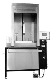
The HAL5224 Hot Air Solder Leveling System is designed to provide the highest quality solder leveling at high throughput rates while preserving the highest reliability and serviceability standards available. Argus International has been designing, building and operating HASL systems for over a decade. The experience earned in a decade of dedication to engineering the HASL process is evident by the high quality work produced.
