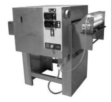
The PC3400 Series flux application systems are designed to support the Argus HAL5224 Hot Air Solder Leveling system by applying flux to circuit boards prior to the HASL process. The PC3400 employs one set of nappy type rollers to provide complete flux coverage. The top roller applies flux to the entire board surface. The bottom roller forces flux into the barrels providing complete surface coverage. Excess flux is filtered and recycled proving a significant cost savings.
