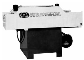
The PC5500 Series precleaning systems were designed to precede Argus the HAL5000 Series Argus Hot Air Solder Leveling systems. The machine is designed to provide a vigorous spray cleaning, fresh water rinse and turbo air dry.
