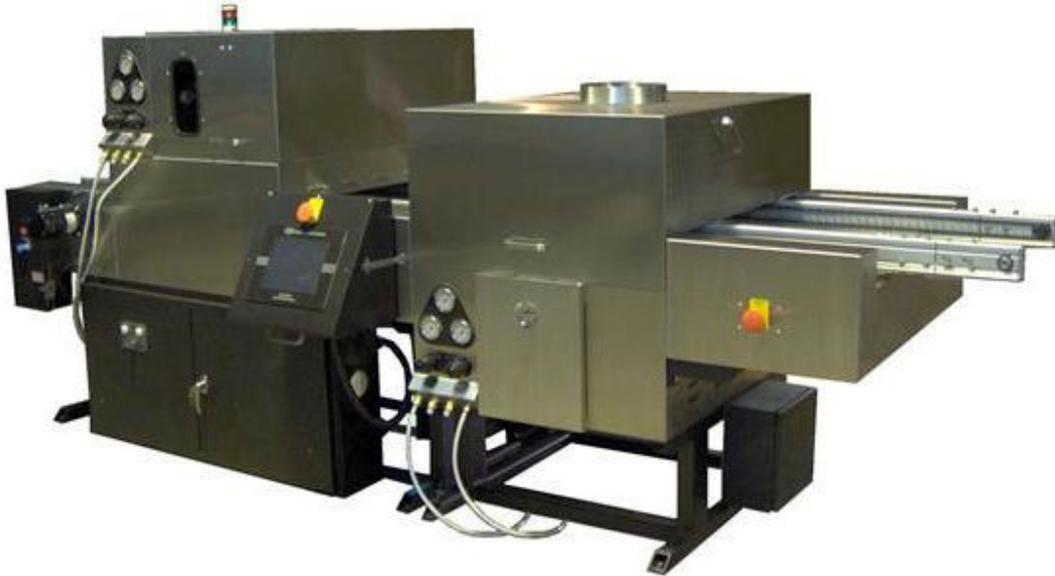
The 9524S (Single-sided) or 9524D (Double-sided) HVLP Spray Units utilize advanced spray technology to apply uniform LPISM coatings to Printed Circuit Boards. This is accomplished by sweeping the heated gun across the PCB at very high speeds as the PCB passes through the spray chamber on a continuously moving edge-contact conveyor. This provides an efficient, reliable system which minimizes over-spray and produces a continuous, conveyORIZED throughput of LPISM-coated boards.
